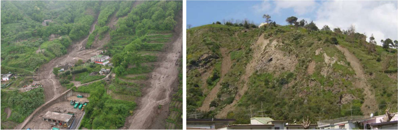
Figure 5: Examples of flow-like mass movements at Monte Vezzi in the Ischia island (2006), on the left, and at Miliscola - Monte di Procida (2010), on the right (both sites are indicated in Fig. 1). (Image credits: Nucleo elicotteri Vigili del Fuoco Salerno; Prof. Paola Romano).
