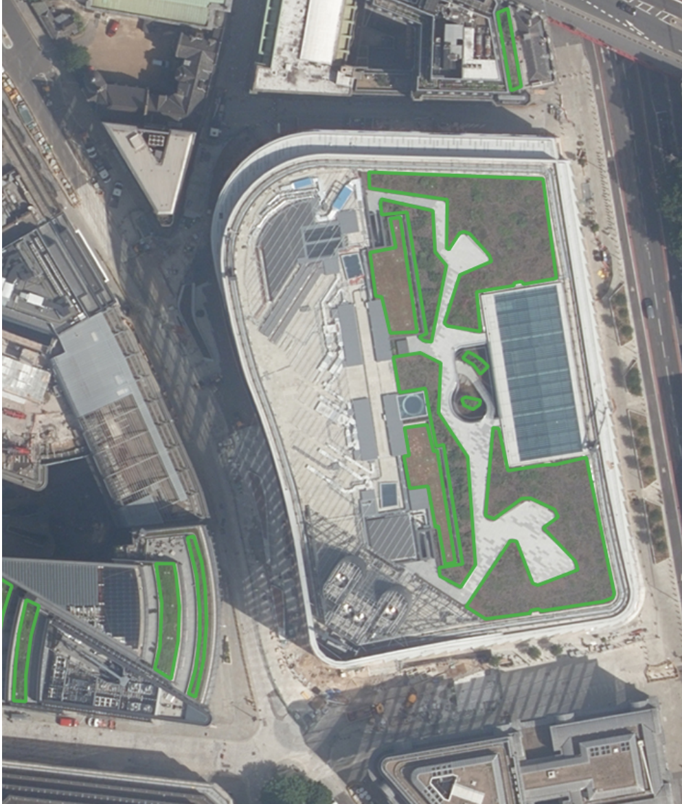
Figure 5. Example of training polygons. The area outlined in green was manually identified as being a green roof in this aerial imagery. Imagery ©GetMapping Plc. Image location is shown in Figure A3.
