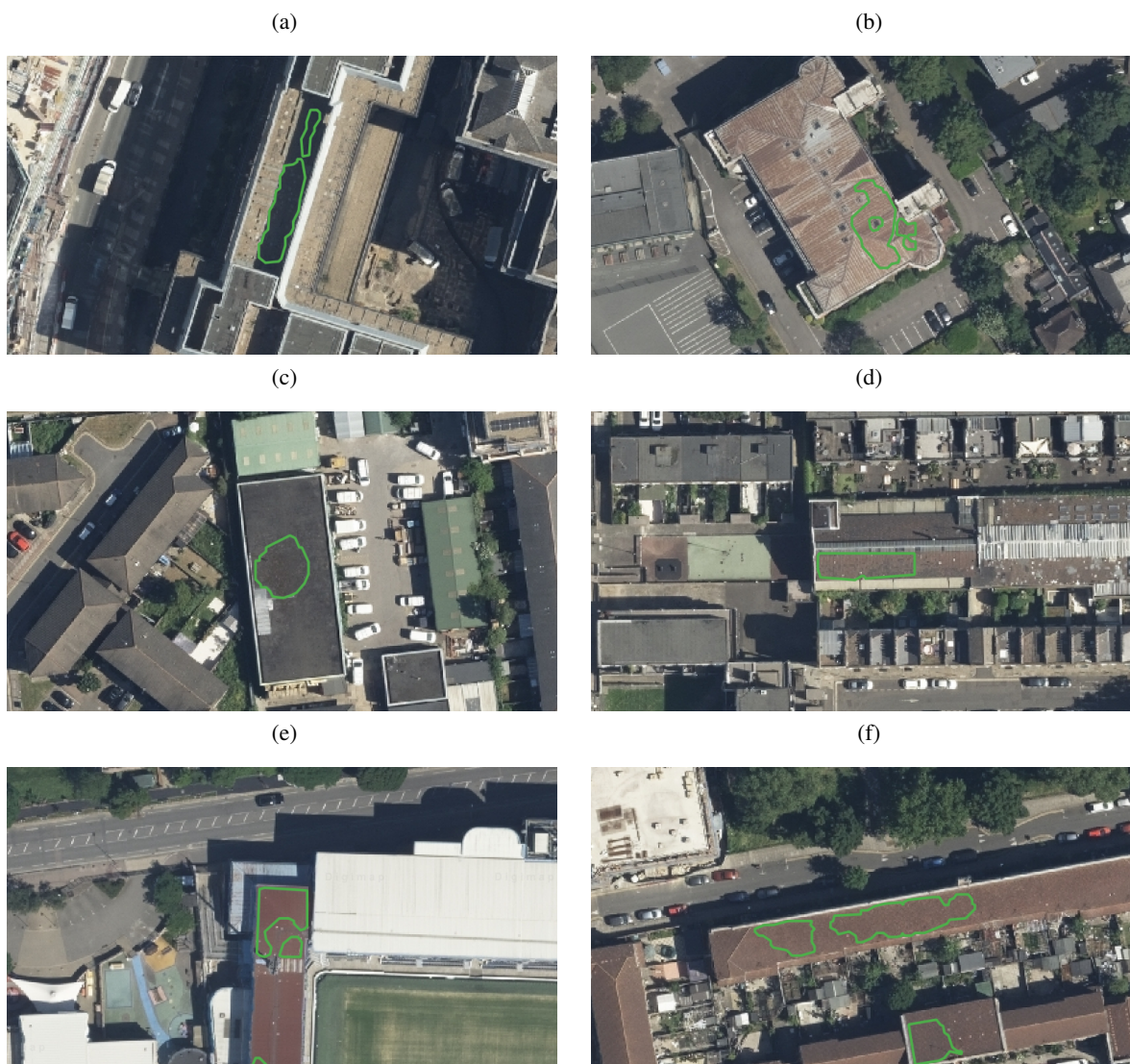
Figure 8. Examples of false positive classification in the 2021 imagery. The green outline shows the area identified as green roof by the model. Imagery ©GetMapping Plc. Image location is shown in Figure A3.
