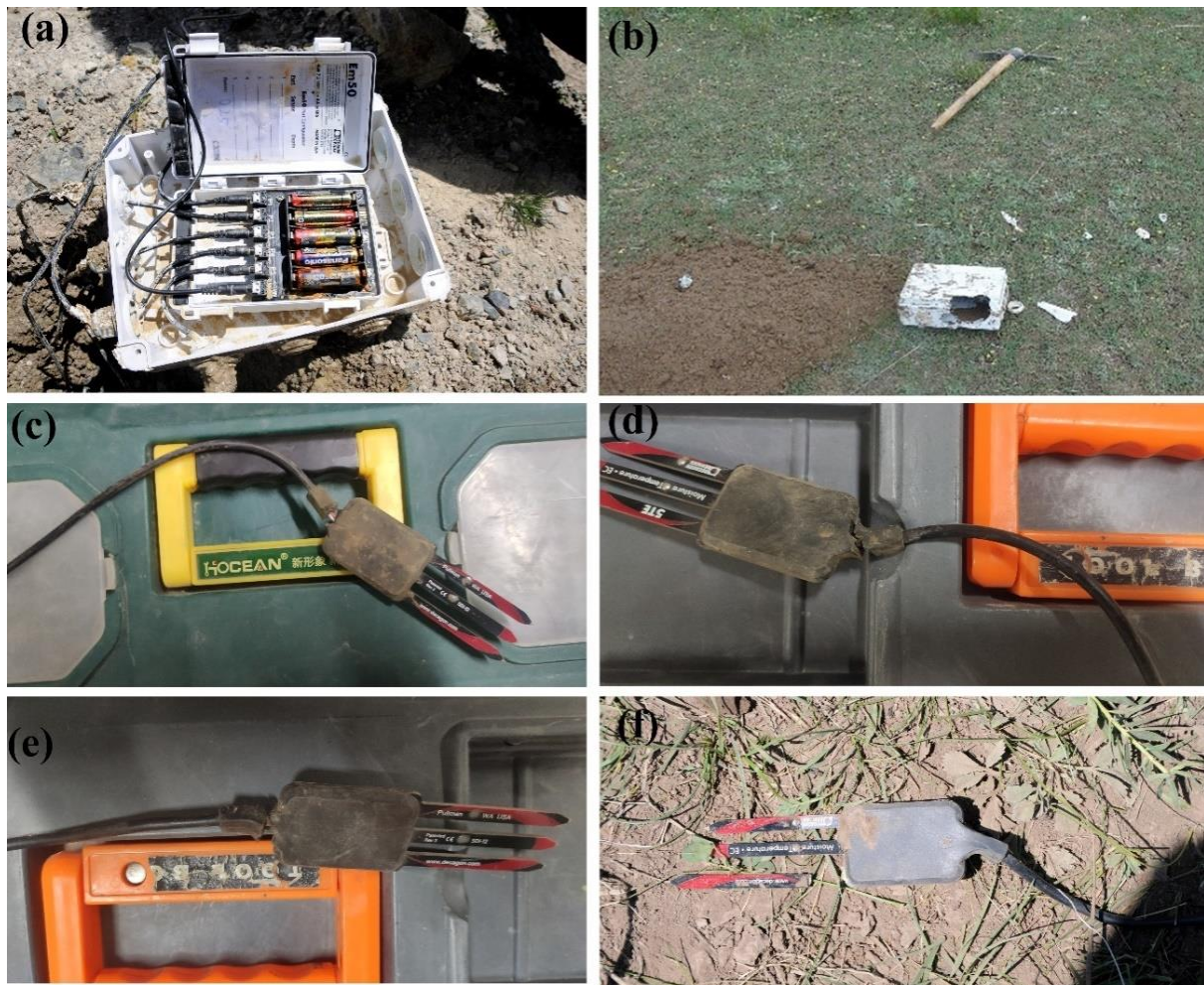
Figure R2. (a) Datalogger damage caused by water ingress, (b) the stolen of 5TE sensor and datalogger in the field (only the broken white waterproof box remains), (c)-(f) the damage of 5TE sensor in the field.
