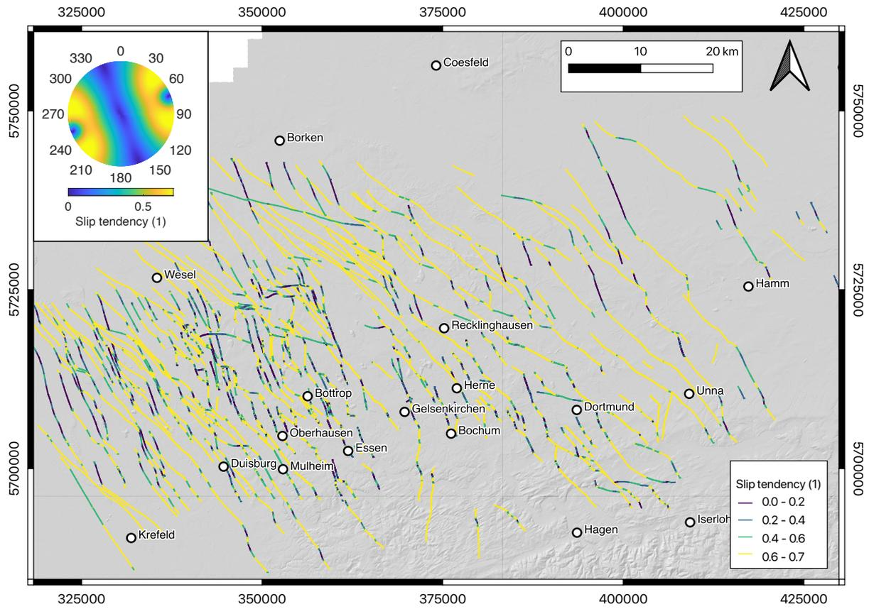
**Fig. 2.** Slip tendency of geological discontinuities within the Ruhr region (GD NRW, 2017) at depth of 1200 m computed based on the stress tensor constrained from this study with  $P_p$  of 11.8 MPa,  $S_{hmin}$  of 17.4 MPa,  $S_{Hmax}$  of 33.7 MPa,  $S_v$  of 29.3 MPa, and average  $S_{Hmax}$  orientation of  $161^\circ$ . Stereographic projection of slip tendency based on the constructed stress tensor is presented in the top left corner.
