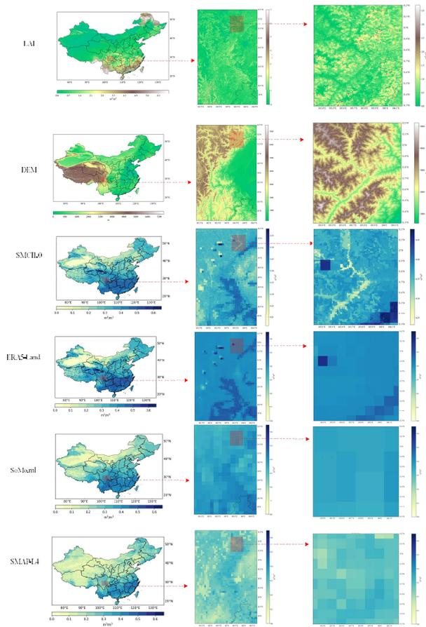
880 **Figure 7:** Soil moisture maps from different products on 1<sup>st</sup> January 2016. The resolution is 1km for SMC1.0, 9km for ERA5-Land and SMAP-L4 and 0.25 degree for SoMo.ml.
