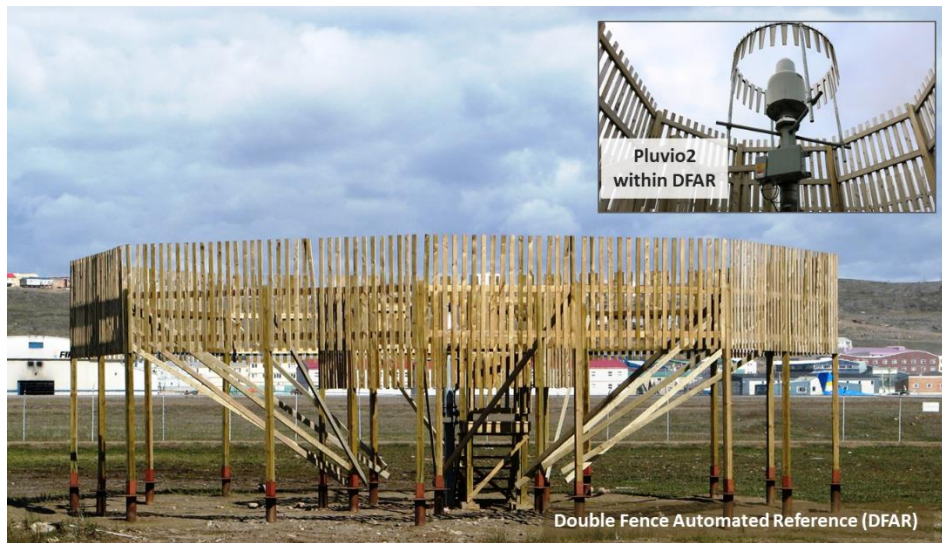
775 Figure 3: Double-fence automated reference (DFAR) configuration at the Iqaluit supersite. Insert: close-up of the single- Alter shielded Pluvio2 precipitation gauge (centre) within inner wooden fence.
