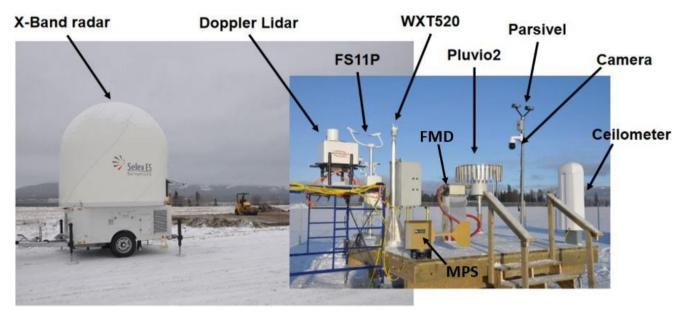
**Figure 5:** The Whitehorse supersite instrument platform and X-band radar (~10 m away) as viewed on December 12 2017. Images were taken facing NE with the CYXY Whitehorse airport runway behind the photographer. All instruments are labelled.
