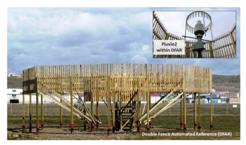
**Figure 3:** Double-fence automated reference (DFAR) configuration at the Iqaluit supersite. Insert: close-up of the single770 Alter shielded Pluvio2 precipitation gauge (centre) within inner wooden fence.
