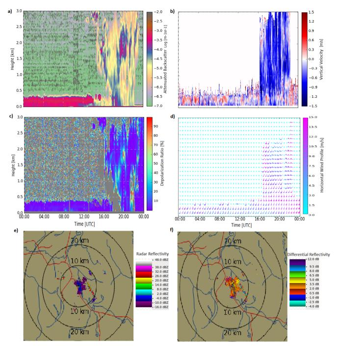
Figure 10: Doppler lidar and X-band radar observations during the HIW event at Whitehorse on December 16 2019. Doppler lidar vertical profiles of (a) attenuated backscatter, (b) vertical velocity, (c) depolarization ratio, and (d) horizontal winds are shown. X-band 3.5° elevation PPI scans of radar reflectivity (e) and differential reflectivity (Z<sub>DR</sub>) (f), provide snapshots of the blizzard in the Whitehorse valley during its peak at 9:45 UTC.
