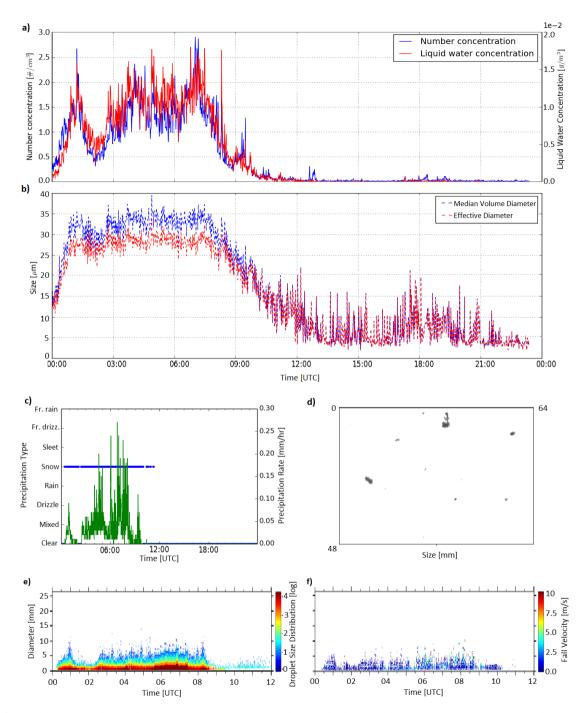
Figure 8: In-situ observations of microphysical properties of precipitation during the November 23 2018 blizzard at Iqaluit:
