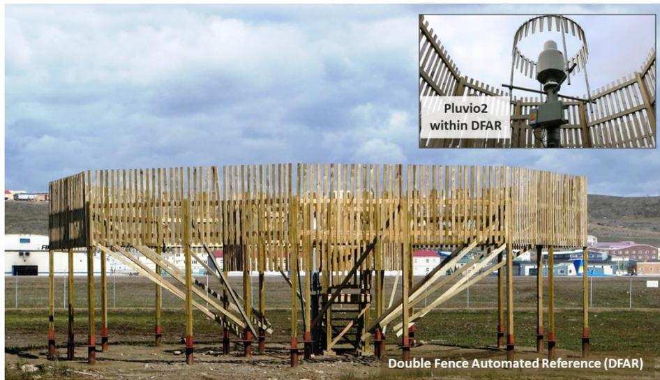
**Figure 3:** Double-fence automated reference (DFAR) configuration at the Iqaluit supersite. Insert: close-up of the single-
