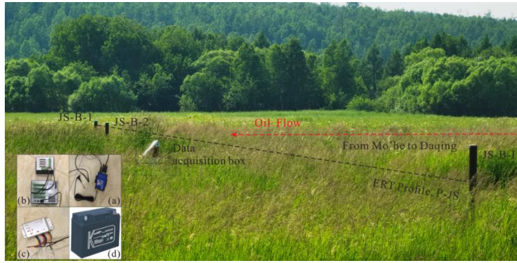
8 Figure S2 Position of boreholes drilled on and off the pipeline ROW and the ERT profile at the JS permafrost site. Photo 9 taken on 29 June 2021. Ground temperatures are measured using thermistor chains connected to the CR3000 data logger. 10 (a) Wireless transmission module (HKT-DTU, Campbell Scientific, Inc., USA), (b) CR3000 data logger with a TRM128 11 multiplexer, (c) Solar charge controller (Phocos ECO (10 A), Germany), (d) Battery cell, a part of the power supply device.
