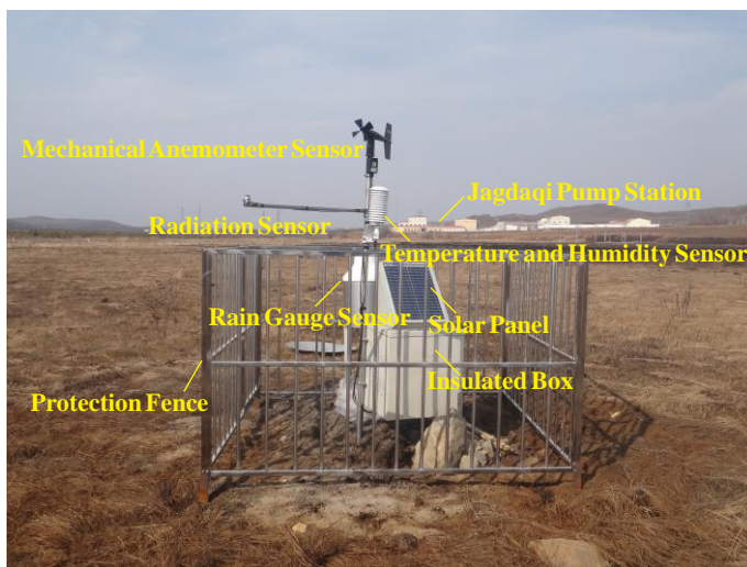
457 458 Figure B1. The automated weather station and instrumentations at the JB site along the China-Russia Crude Oil Pipelines 459 route in the northern Da Xing'anling Mountains, Northeast China. Notes: Photo was taken on April 2018. The rain gauge 460 sensor has been installed but is ineffective. The photo shows the location of the Jagdaqi pump station. The CR3000 data 461 logger, multiplexer, battery cell, solar charge controller, and wireless transmission module are placed in the white box 462 with a solar panel ( i.e. , insulated box). All monitoring devices are protected by an aluminum alloy fence.
