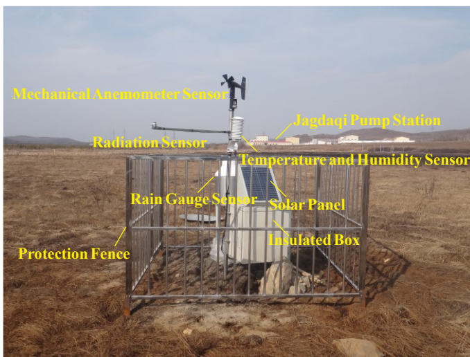
501 502 Figure B1. The automated weather station and instrumentations at the JB site along the China-Russia Crude Oil Pipelines 503 route in the northern Da Xing'anling Mountains, Northeast China. Notes: Photo was taken on April 2018. The rain gauge 504 sensor has been installed but is ineffective. The photo shows the location of the Jagdaqi pump station. The CR3000 data 505 logger, multiplexer, battery cell, solar charge controller, and wireless transmission module are placed in the white box 506 with a solar panel ( i.e. , insulated box). All monitoring devices are protected by an aluminum alloy fence.
