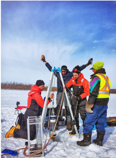
Figure E1. Picture taken during Leg 1 of the Nunataryuk expeditions showing the setup of the tripod and corer (Picture by Martine Lizotte).
