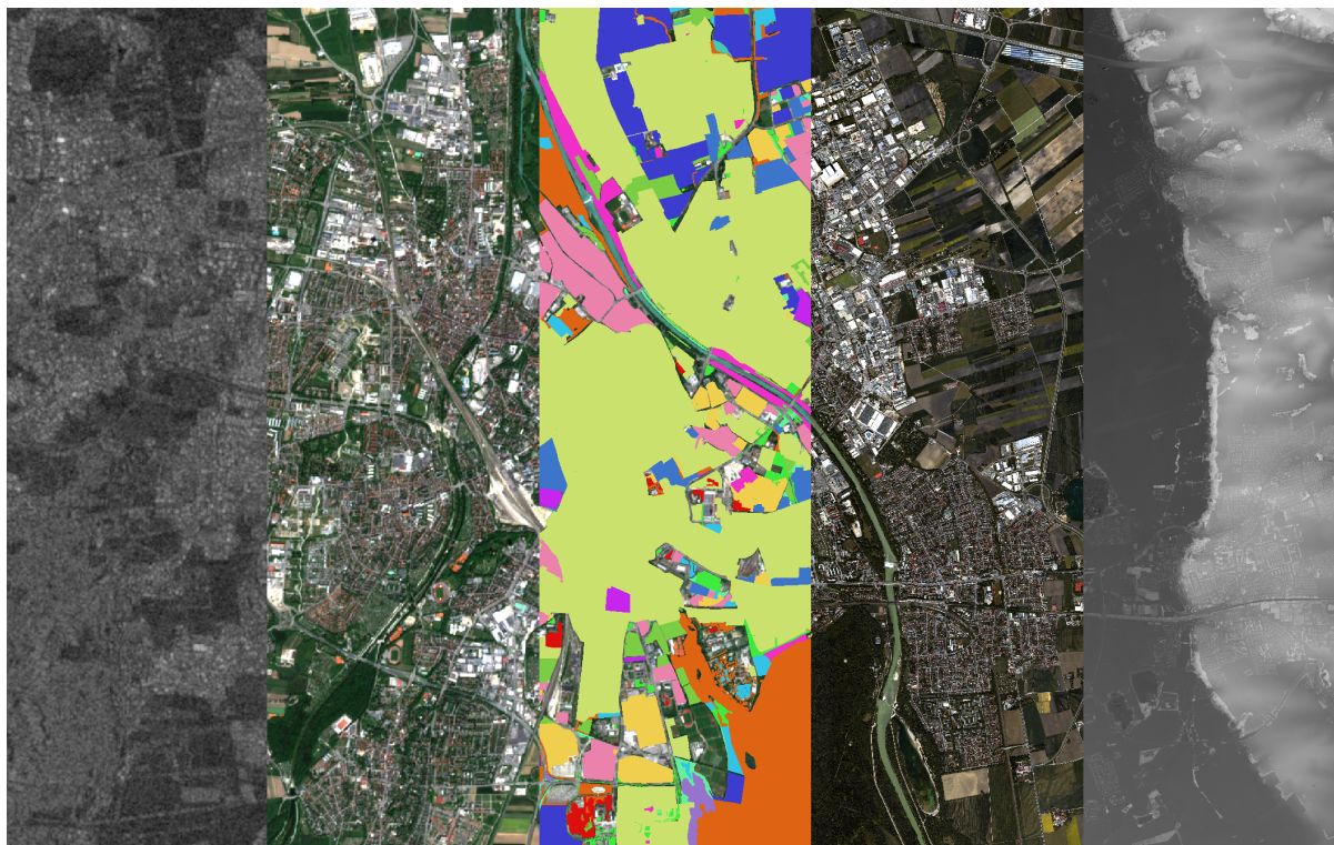
Figure 1. The Visualization of five data modalities in MDAS. From left to right: the Sentinel-1 image (VH band in dB), the Sentinel-2 image (RGB: 665 nm, 560 nm, 490 nm), the OSM land use layer, the HySpex image (RGB: 691 nm, 569 nm, 445 nm), and the DSM.
