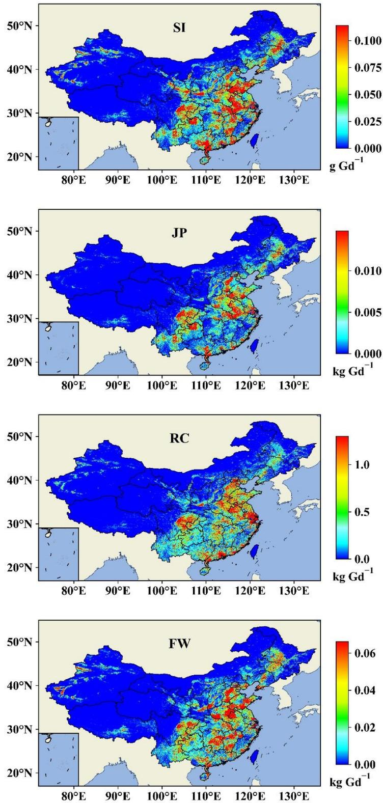
**Figure S10** Distribution of OC emission from different sources in 2018. Colorbar shows the emissions in each grid.
