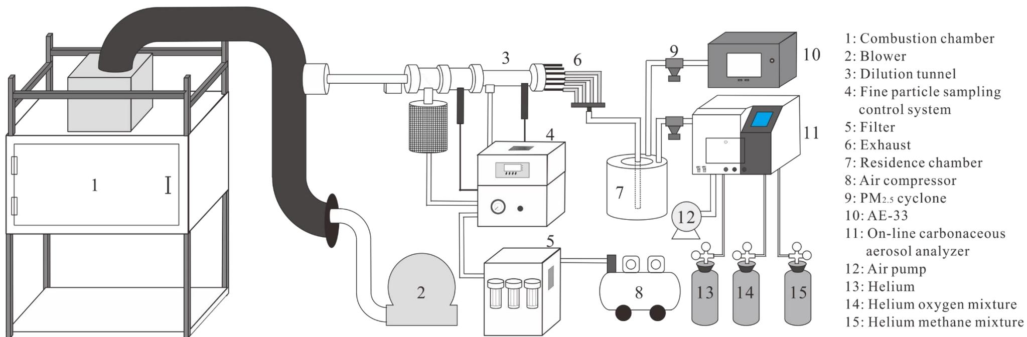
**Figure S2** Structure of the combustion and dilution sampling system adopted in this study
