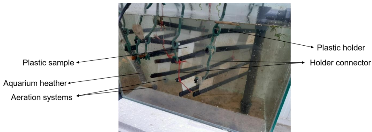
130 Figure 1. Aquarium set-up for biofilm growth on pristine plastic specimens. Picture taken by Giulia Leone
