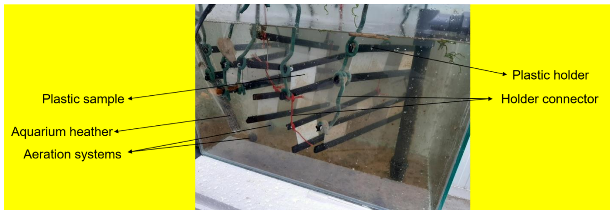
130 Figure 1. Aquarium set-up for biofilm growth on pristine plastic specimens. Picture taken by Giulia Leone
