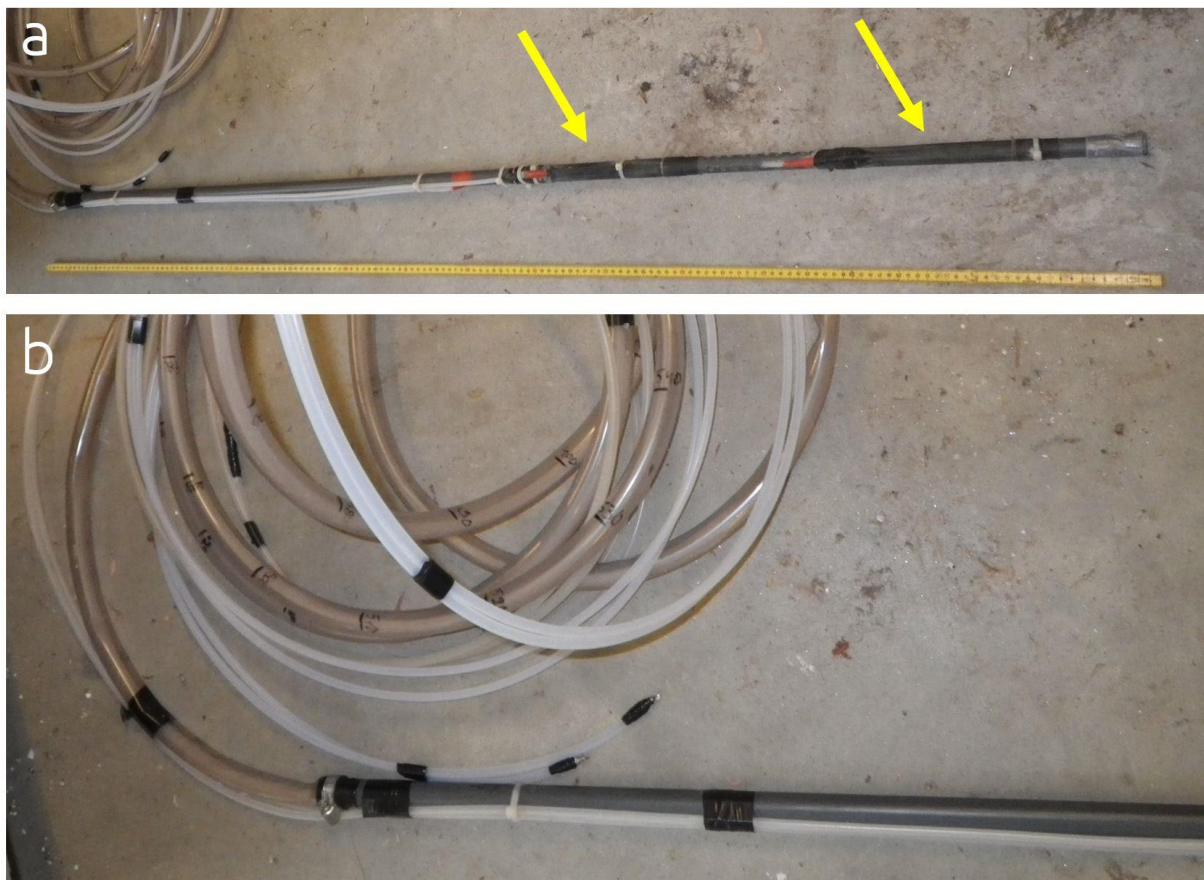
770 Figure A 3: Photo of the custom-made straddle packer system with two inflatable parts to isolate specific depths in the wells and to pump water from specific depth (a) and the upper part and tubing system (pumping tube and two air tubes to inflate the flexibles tube parts) of the packer system (b). The yellow arrows in (a) indicate inflatable packer system parts to seal off the water above and below the selected sample depth.
