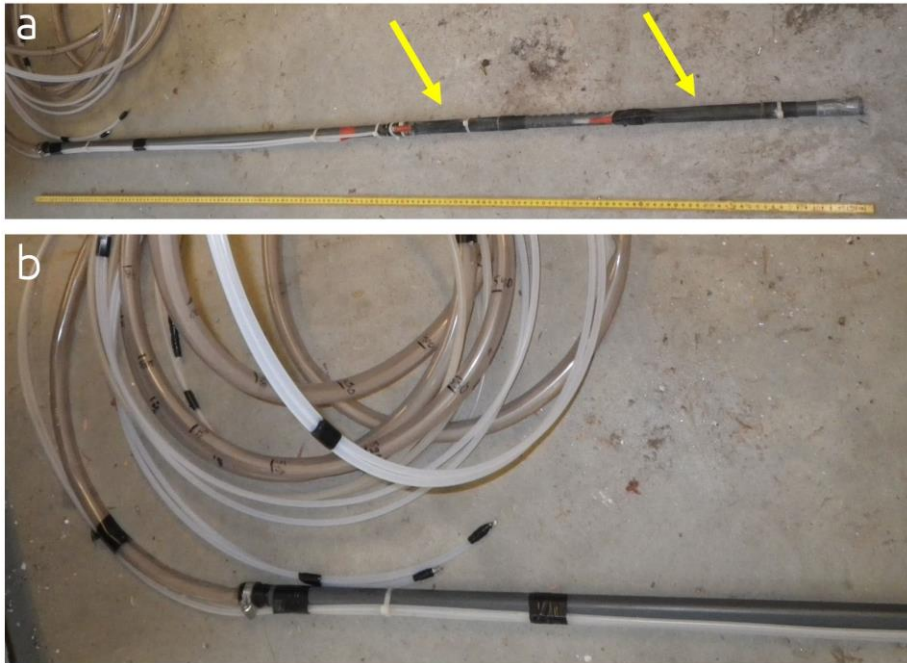
900 Figure A 3: Photo of the custom-made straddle packer system with two inflatable parts to isolate specific depths in the wells and to pump water from specific depth (a) and the upper part and tubing system (pumping tube and two air tubes to inflate the flexible tube parts) of the packer system (b). The yellow arrows in (a) indicate inflatable packer system parts to seal off the water above and below the selected sample depth.
