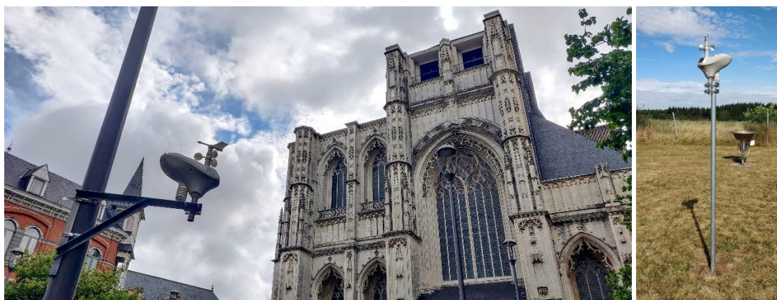
Figure 1: The outdoor unit of the WH2600 wireless digital weather station at the Mathieu Layensplein in Leuven (LC-105) (a) and next to the official AWS equipment in Humain (LC-R05) (b). Pictures: Maarten Reyniers.
