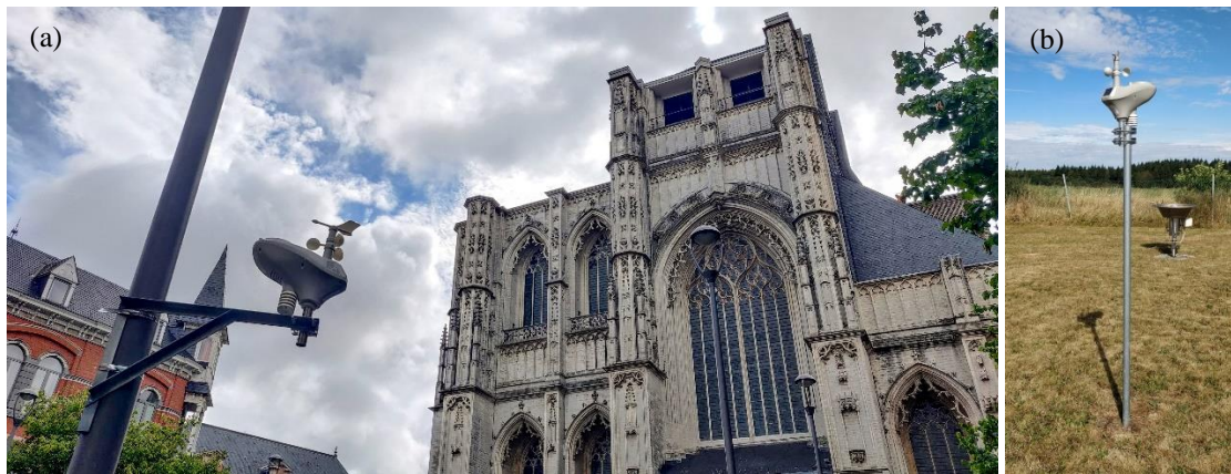
155 Figure 1: The outdoor unit of the WH2600 wireless digital weather station at the Mathieu Layensplein in Leuven (LC-105) (a) and next to the official AWS equipment in Humain (LC-R05) (b). Pictures: Maarten Reyniers.
