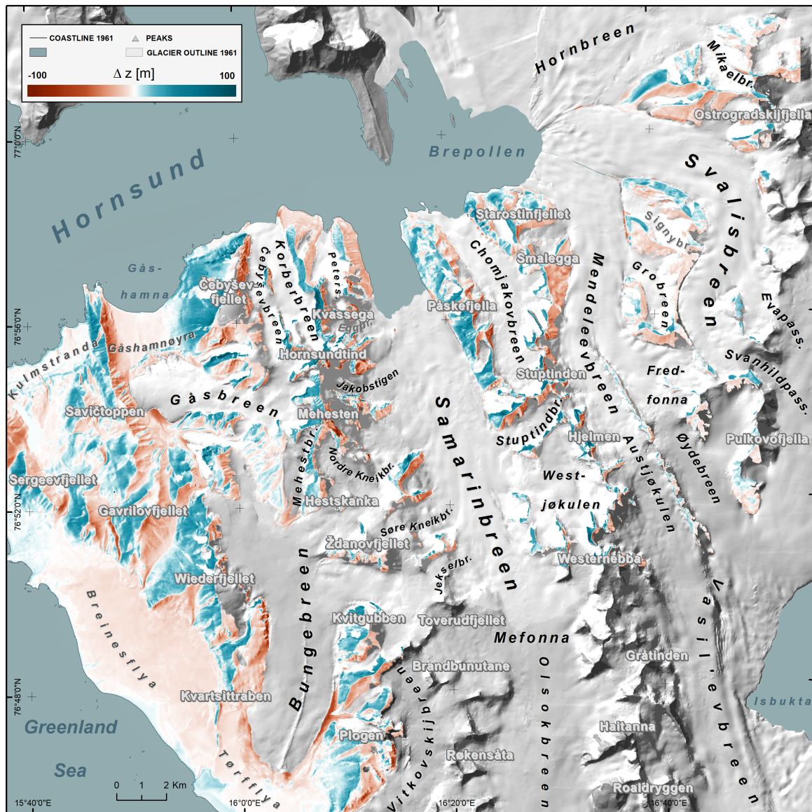
Figure 8. Elevation differences between the 1961 DEM generated from IGF PAN maps issued in 1987 (map rectification based on the nodes of the cartographic grid) and the 2010 DEM generated by NPI (2014).
