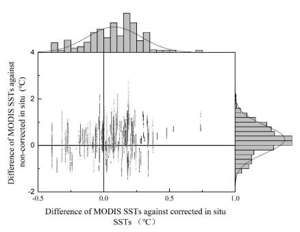
605 Figure 13. Marginal Histogram of the difference between in situ data before and after correction and the corresponding MODIS SST data. (The margins of the scatterplot is a histogram of the variables, indicating the distribution of data in either direction)
