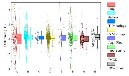
Figure 6. Box chart with scatters representing the differences between the original MODIS data and eight types of in situ 340 SST observations.
