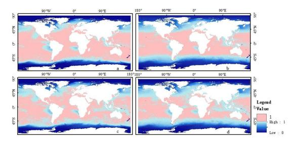
Figure 7. Frequency of nonnull pixels, including valid pixels and low-quality pixels, in the monthly MODIS SST data during the study period from (a) nighttime Aqua overpasses, (b) daytime Aqua overpasses, (c) nighttime Terra overpasses, and (d) daytime Terra overpasses.
