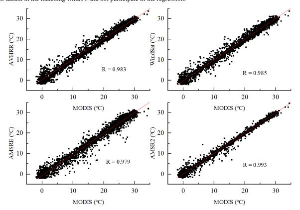
Figure 5. Scatter diagrams of the MODIS SST data and ocean multisource data compensated for different measurement times
