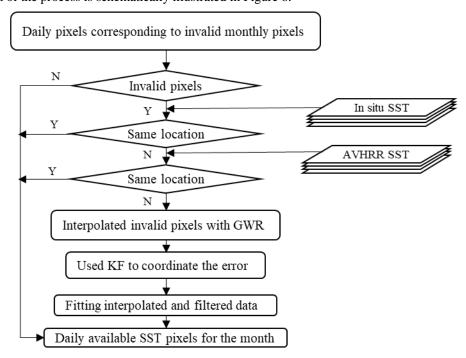
Figure 8. A summary flowchart for reconstructing invalid SST pixels in the marginal low- and mid-latitude regions Invalid pixels were filled with in situ or AVHRR SST data at the same location and time (priority was given to the use of
