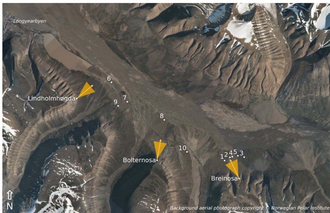
Figure 1: Locations of the instrumentation in the valley of Adventdalen in 2018 (white dots). The racks are labeled with their respective number and the landscape cameras are labeled according to the nearby mountain peak. The yellow arrows show the direction in which the landscape cameras are pointed, and the triangles show their approximate viewing angle. The background image is a composite of several aerial photographs taken in July 2009, used with courtesy of the Norwegian Polar Institute.
