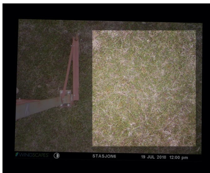
Figure 3. Example of a stabilized photo from rack 6, taken on the 19 th of July 2018 at noon. Slight movements by the thawing of the topsoil turned this camera a few angles out of its original position, which was corrected for by the stabilization algorithm through a rotation of the photo. The bright rectangle indicates the mask for which the greenness index was calculated, which excludes parts of the photo where the rack itself is visible as well as areas where shadows were cast by the rack (darkened regions). The ground surface defined by these masks has been verified to be visible in all photos.
