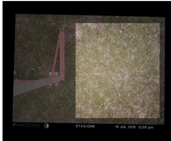
Figure 3. Example of a stabilized photo for rack 6, taken on the 19 th of July 2018 at noon. Slight movements by the thawing of the topsoil turned this camera a few angles out of its original position, which was corrected for by the stabilization algorithm through a rotation of the photo. The bright rectangle indicates the mask for which the greenness index was calculated, which excludes parts of the photo where the rack itself is visible as well as areas where shadows were cast by the rack (darkened regions). The ground surface defined by these masks has been verified to be visible in all photos.
