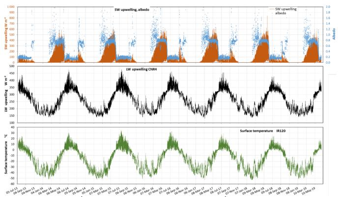
390 Figure 6. Time series of SW↑ radiation from the CNR4 radiometer, albedo, LW↑ radiation from the CNR4 radiometer and surface temperature from the IR 120 infrared sensor. The albedo values are shown with a reversed scale to minimize overlap with the SW↑ plot. Most albedo values over snow-covered surfaces that are very different from 0.8 are due to the use of ERA5 SW↓ values.
