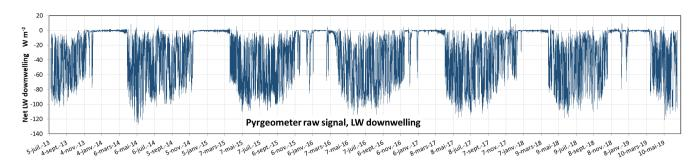
Figure 4. Raw longwave downwelling radiation measured by the CNR4. The near-zero values in winter over extended periods indicate the presence of frost on the pyrgeometer window. The data for those periods are thus invalid.
