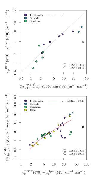
Figure 6. Evaluation of  $c_p$  measurement bias due to the finite acceptance of the spectrophotometer. (A) Relation between the difference of the  $c_p$  measured with the spectrophotometer and the LISST, and the VSF integral in the range of solid angles defined by the difference of their acceptance angles. (B) Relation between the scattering coefficient ( $b_p = c_p - a_p$ ) and the magnitude of scattering between 0.018° and 0.074° scattering angles ( $\psi$ ).
