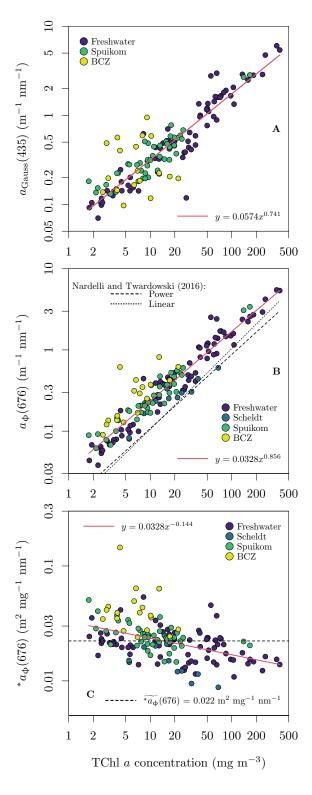
Figure 5. Relation between the total chlorophyll a (monovinyl chlorophyll a + chlorophyllide a) and in vivo pigment absorption. (A) Magnitude of the Gaussian peak centered at 435 nm: (B) the in vivo pigment absorption at 676 nm,  $a_{\Phi}(676)$ ; and (C) mass-specific in vivo pigment absorption at 676 nm,  $*a_{\Phi}(676)$ . The  $a_{\Phi}(676)$  for the Scheldt samples were estimated as the  $a_{nw}(650, 676, 715)$  line height (Roesler and Barnard, 2013).
