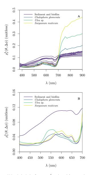
Figure 10. Lambert-equivalent substrate bi-hemispherical reflectance,  $\rho_s^L$ , estimated from samples on the Spuikom. The view geometry was nadir view ( $\theta=0^{\circ}$ ,  $\Delta\phi$  undefined) for all measurements. (A) The magnitude of  $\rho_s^L$  in the visible to NIR spectral range and (B) the magnitude in the visible spectral range. In (B) only the sediment samples with the thinnest and thickest biofilm mats are shown, as judged by the reflectance magnitude at 676 nm.
