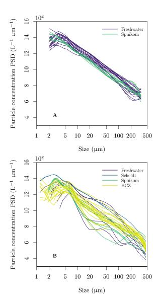
**Figure 12.** Particle size distribution (PSD) in the Belgian water systems. (A) Retrieved with the LISST-100X; and (B) retrieved with the LISST-200X. The continuous particle number concentration PSD was calculated from the volume concentration PSD assuming spherical particles of median diameter in each size bin and normalizing by the width of each logarithmically spaced size bin.
