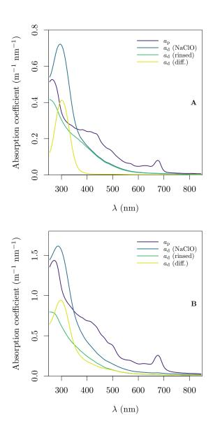
Figure 2. Evaluation of the treatment of the filters with sodium hypochlorite (NaClO) and subsequent rinse on the determinations of  $a_d$ . (A) A sample from the Bocht (BL\_08) and (B) a sample from the Dikkebus (DK\_01). The sample in (B) show loss of absorbing material after rinsing.
