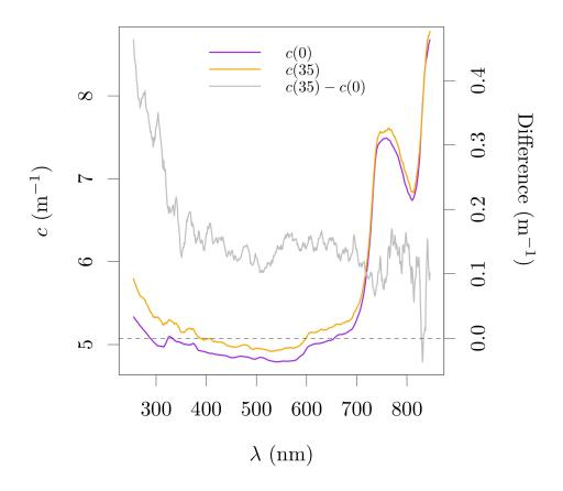
Detailed example of the validation of the particle beam attenuation coefficient,  $c_p$ , measured with the spectrophotometer at an acceptance angle of 0.074° against the values measured by the LISST instruments at an acceptance angle of 0.018°. The difference between  $c_p$  measured by the different instruments (A) is accounted by the scattering within the difference of acceptance angle of the instruments, as estimated from the particle volume scattering function,  $\beta_p$  (B).
