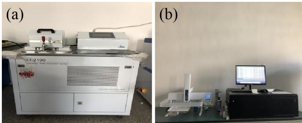
Figure. C3 Analytical instruments. (a) Li-2100 Automatic Vacuum Condensation Extraction instrument, (b) LWIA-24D Liquid water isotope Analyzer.
