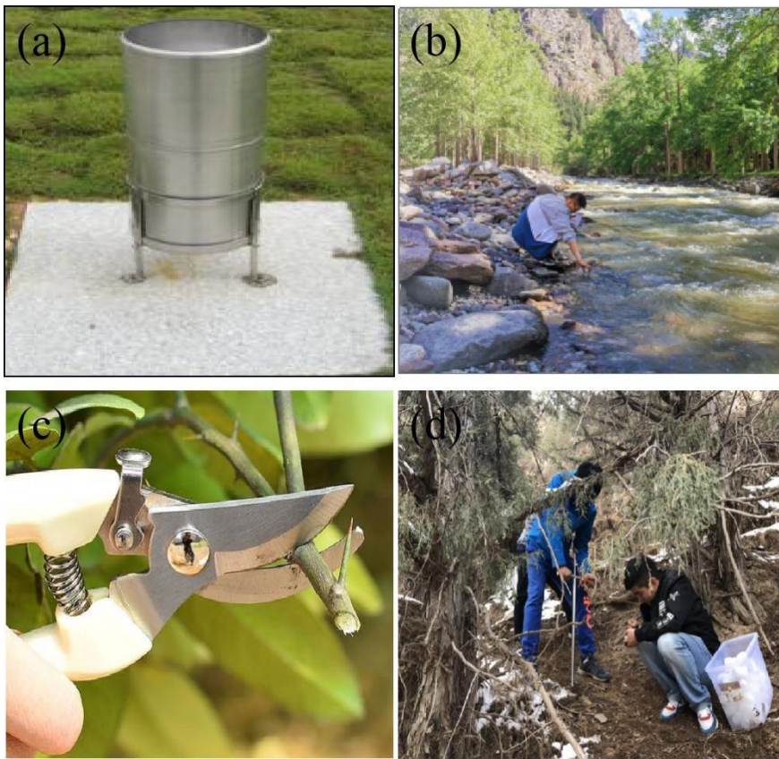
Figure. C2 Sampling instruments. (a) Rain gauge collecting precipitation, (b) surface water sampling, (c) sampling shears collecting vegetation stems, and (d) earth drill collecting soil samples.
