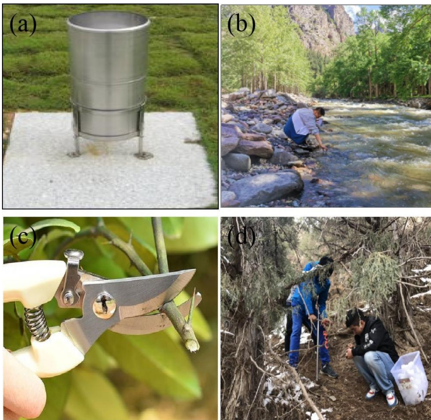
315 Figure. C2 Sampling instruments. (a) Rain gauge collecting precipitation, (b) surface water sampling, (c) sampling shears collecting vegetation stems, and (d) earth drill collecting soil samples.
