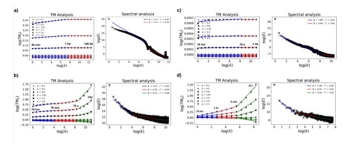
**Figure 9.** TM analysis (Eq. 4 in log-log plot), and spectral analysis (Eq. 3 in log-log plot) of 1 month long data (27/01/2021 to 27/02/2021) for a) anemometer data at 100 Hz (sample length of 40 min), b) fluctuations of anemometer data at 1 Hz (sample length of 16 hours), c) Temperature (*T*) at 1 Hz (sample length of 16 hours), d) fluctuations of Temperature (*T*) at 15 s (sample length of 16 hours)
