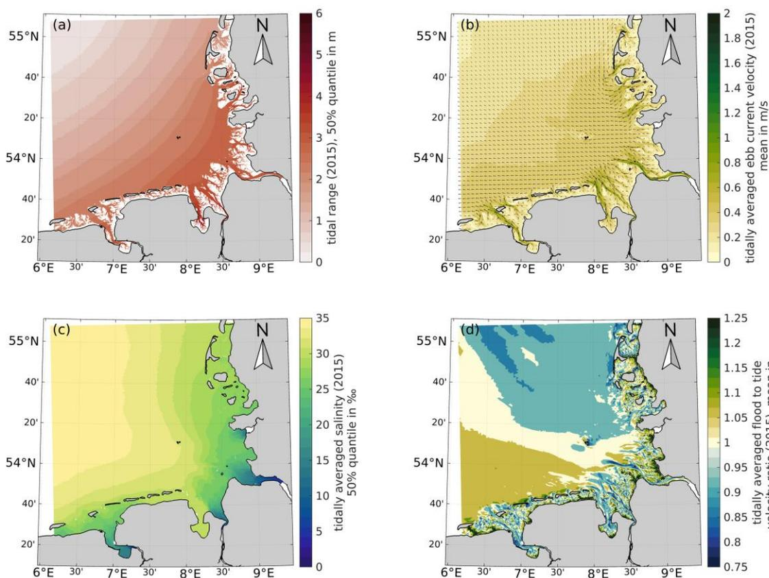
280 **Figure 8: Examples of tidal characteristic values for 2015: (a) 50% quantile of tidal range in m, (b) mean, tidally averaged ebb current velocity in m/s, (c) mean salinity in ppt and (d) ratio of mean flood and mean tidal current velocity in -.**
