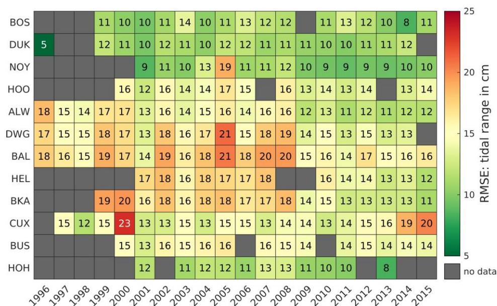
335 **Figure 10: Root mean square error (RMSE) of the tidal range in cm between 1996 to 2015 at representative gauges.**
