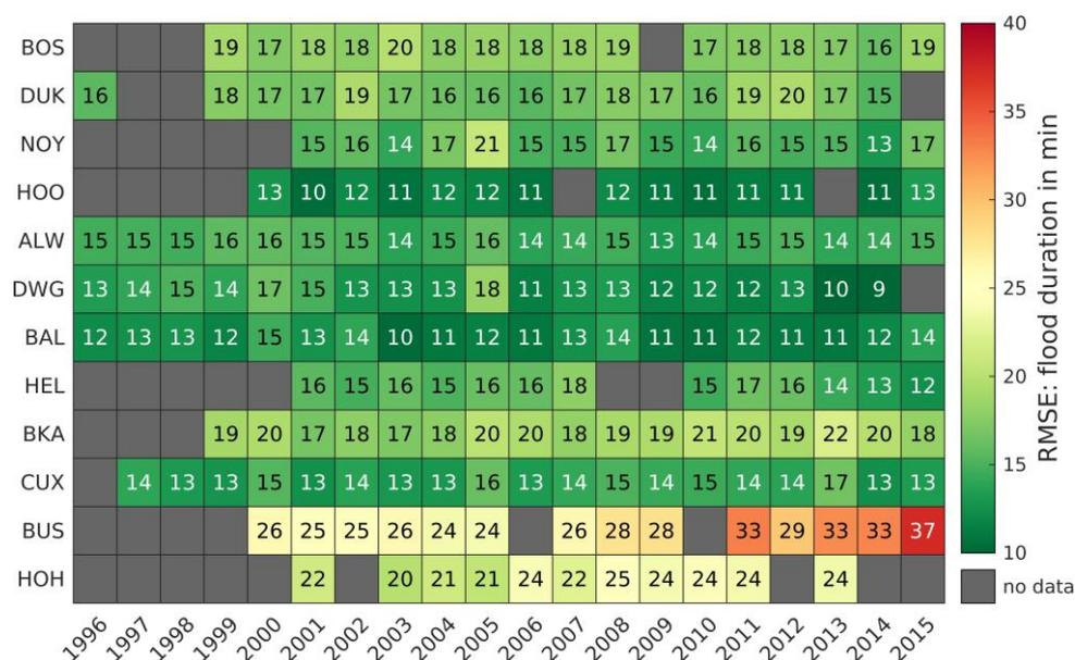
365 **Figure 12: Root mean square error (RMSE) of the flood duration in minutes between 1996 and 2015 at representative gauges.**
