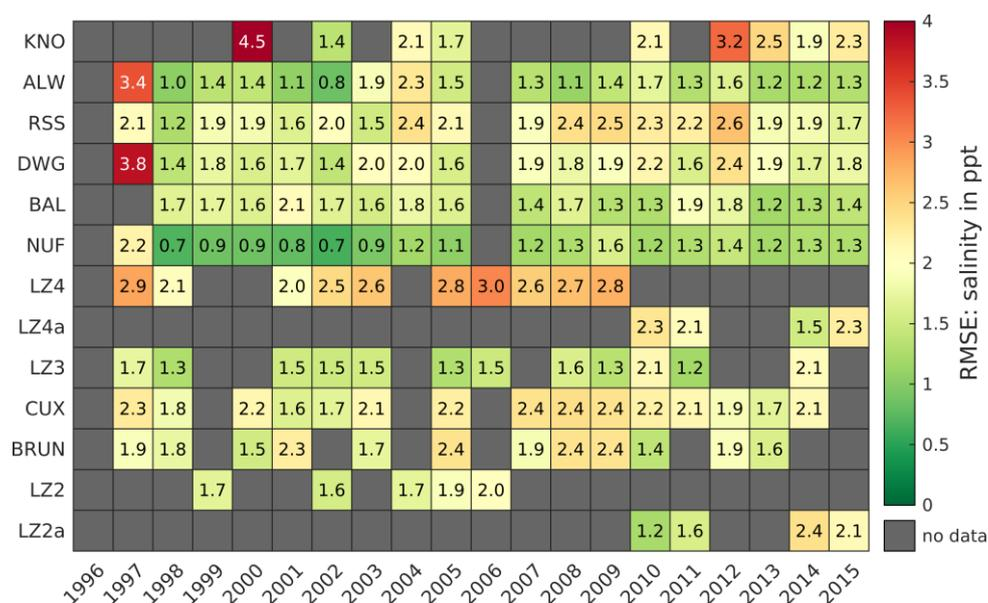
Figure 14: Root mean square error (RMSE) of the salinity in ppt between 1996 and 2015 at representative gauges.
