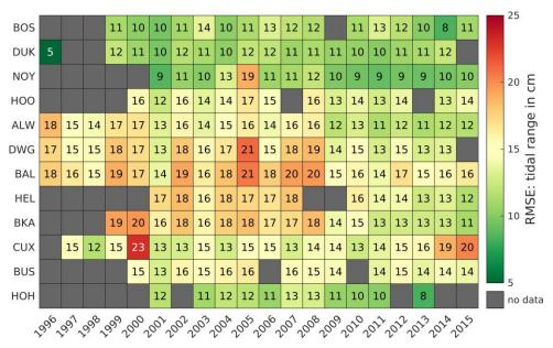
Figure 10: Root mean square error (RMSE) of the tidal range in cm between 1996 to 2015 at representative gauges.
