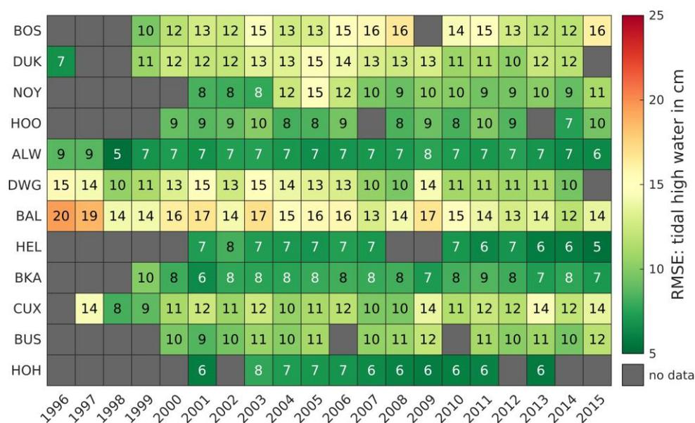
355 **Figure 11: Root mean square error (RMSE) of the tidal high water in cm between 1996 and 2015 at representative gauges.**
