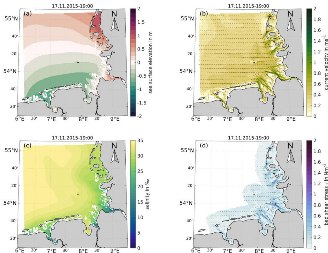
**Figure 6: Exemplary hydrodynamic state on 17. November, 2015 7:00 PM, showing sea surface elevation (a) in mNHN, current velocity magnitude and direction (b) in m/s, salinity (c) in ppt and bottom shear stress magnitude and direction (d) in  $N/m^2$ .**
