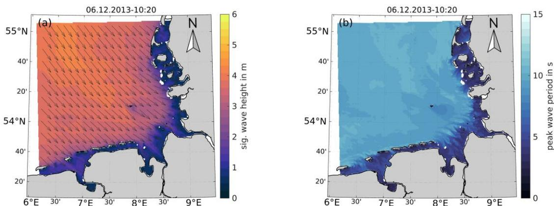
250 **Figure 7: Exemplary wave state during a storm “Xaver”, in 2013 showing significant wave height  $h_{m0}$  in meters, the mean wave direction  $\Theta_m$  (a) and peak wave  $T_p$  period in seconds (b) in the EPZ. Note that the mean wave direction vectors in (a) are normalized.**
