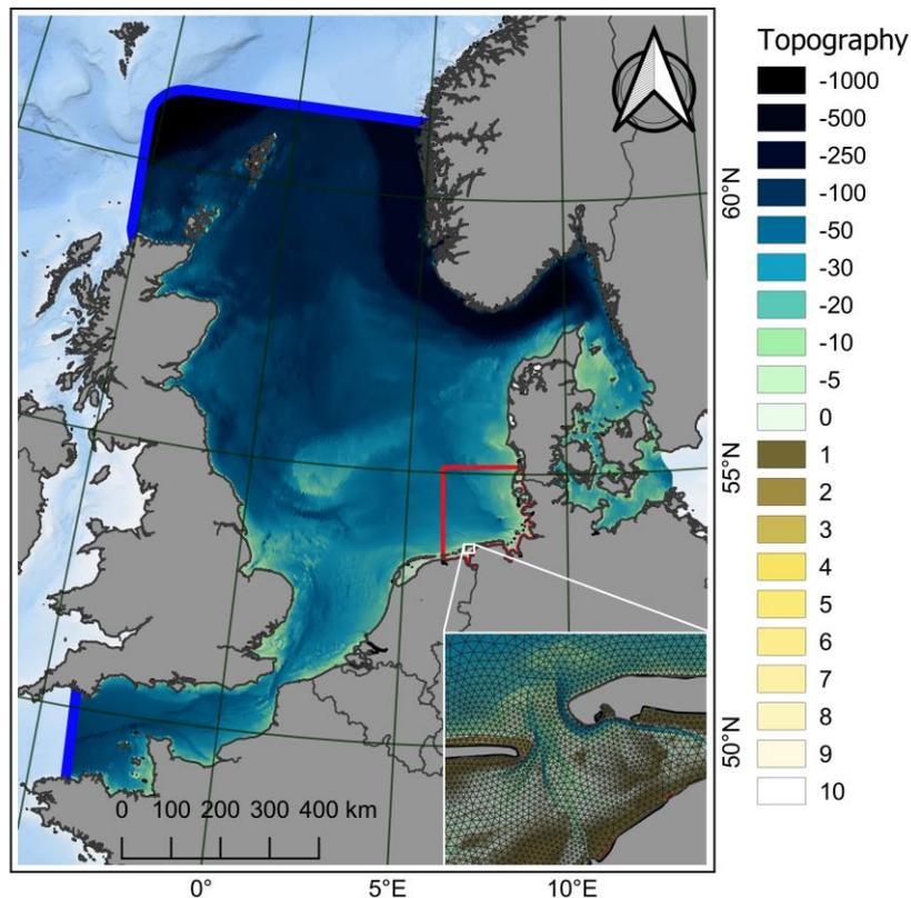
155 **Figure 3:** The grid of the numerical North Sea model showing the grid in grey, the open boundaries in blue, the EasyGSH-DB
