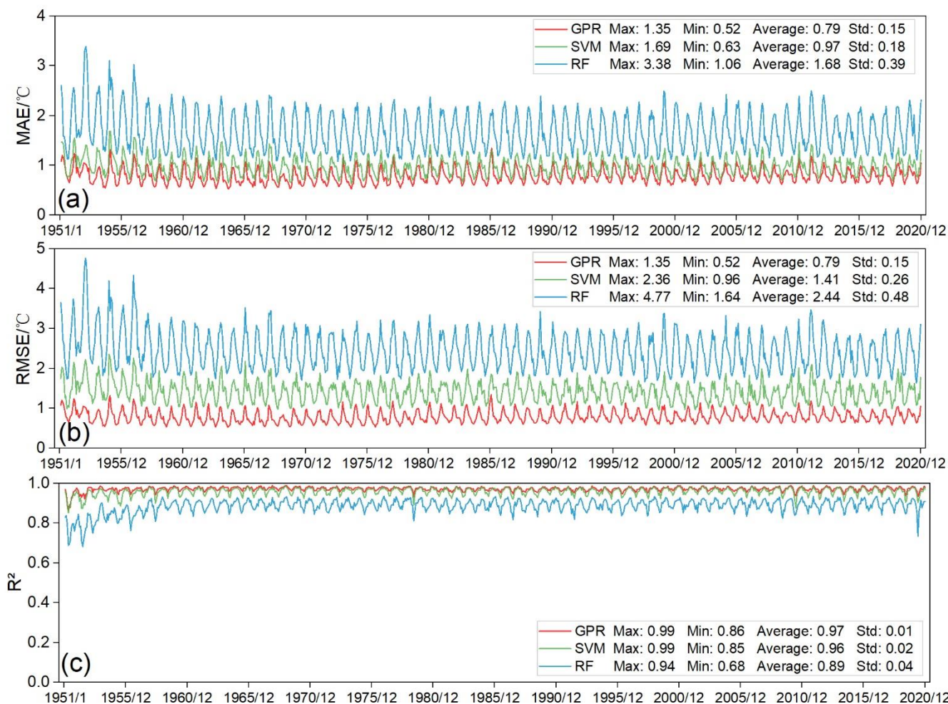
Figure 3: (a) Mean absolute error (MAE), (b) root mean square error (RMSE), and (c) coefficient of determination ( R^2 ) between observed Tmean and predicted Tmean by the three machine learning models (GPR, SVM, RF) of the test meteorological stations over the period from January 1951 to December 2020. See Figure S4 and Figure S5 for the accuracy graph of Tmax and Tmin.
