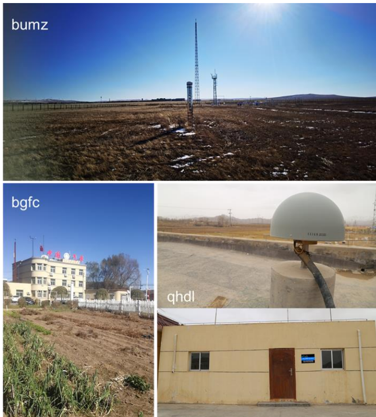
Figure 5. Photos of typical GNSS sites. “bumz” and “bgfc” are two high-quality CMA sites, and “qhdl” is a low- 290 quality CEA site that is not suitable for snow depth retrieval.
