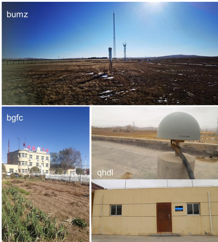
Figure 5. Photos of typical GNSS sites. “bumz” and “bgfc” are two high-quality CMA sites, and “qhdl” is a low-quality CEA site that is not suitable for snow depth retrieval.
