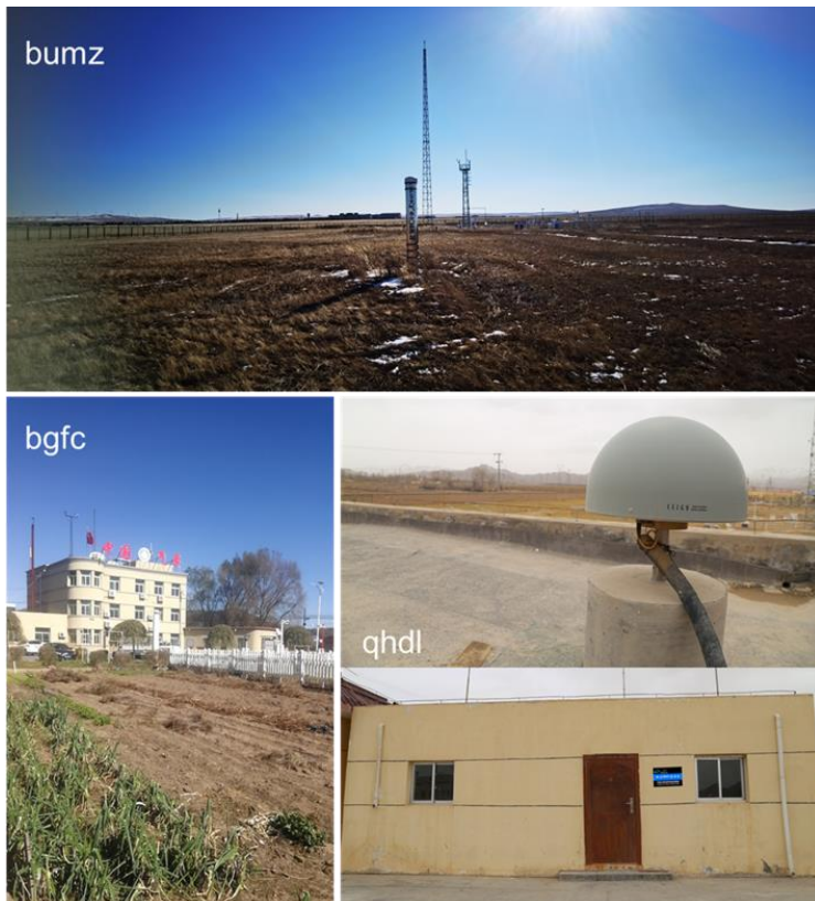
285 Figure 5. Photos of typical GNSS sites. “bumz” and “bgfc” are two high-quality CMA sites, and “qhdl” is a low-quality CEA site that is not suitable for snow depth retrieval.
