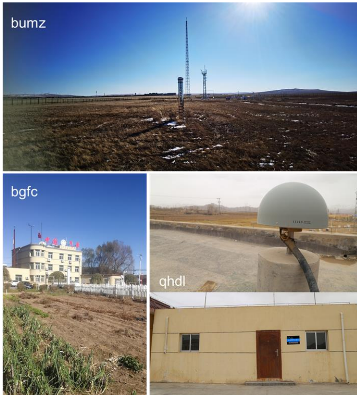
305 Figure 5. Photos of typical GNSS sites. “bumz” and “bgfc” are two high-quality CMA sites, and “qhdl” is a low-quality CEA site that is not suitable for snow depth retrieval.
