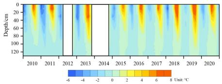
**Figure 4.** Active layer soil temperature profiles during 2010-2020 at the Mahan Mountain permafrost site. The blank gap stands for the major missing data from 21 March 2012 to 9 September 2012, and from 23 November 2013 to 21 September 2014, respectively.
