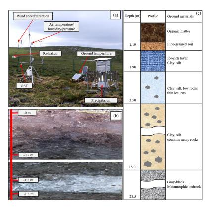
**Figure 2.** The setup of the meteorological and permafrost observation site in the Mahan Mountain. The meteorological monitoring parameters mainly includes: wind speed and direction, air humidity, radiation, ground surface temperature (GST) and precipitation (a); active layer soil profile and ground ice near permafrost table (b); soil profiles information of the permafrost borehole (c).
