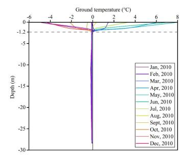
Figure 7. Ground temperature envelopes in the permafrost borehole drilled in 2010 at the Mahan
