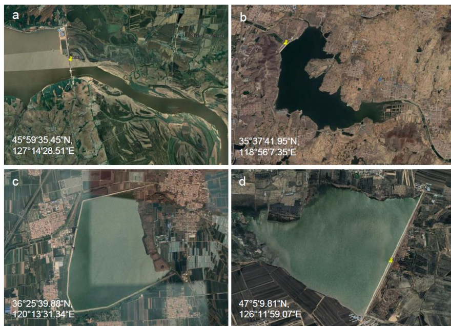
Fig. S1. Types of dams/reservoirs in this study. (a-b) On-stream dam/reservoir constructed on a river/stream regardless of impoundment; (c-d) Off-stream dam/reservoir formed by partial or complete embankment around an off-stream lake. The high-resolution images in this figure were from the Google Earth Pro.
