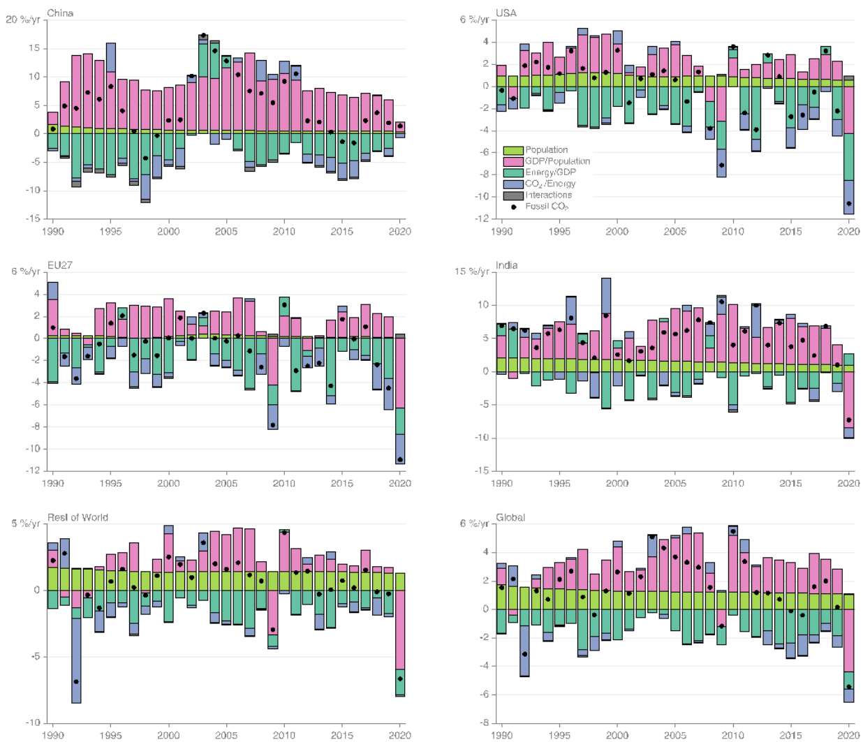
Figure 14. Kaya decomposition of the main drivers of fossil CO 2 emissions, considering population, GDP per person, Energy per GDP, and CO 2 emissions per energy, for China (top left), USA (top right), EU27 (middle left), India (middle right), Rest of the World (bottom left), and World (bottom right). Black dots are the annual fossil CO 2 emissions growth rate, coloured bars are the contributions from the different drivers. A general trend is that population and GDP growth put upward pressure on emissions, while energy per GDP and more recently CO 2 emissions per energy put downward pressure on emissions. The changes during 2020 led to a stark contrast to previous years, with different drivers in each region.
