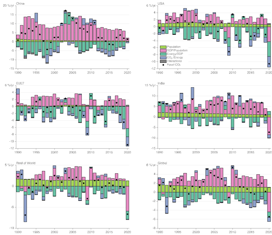
13.18 Figure 14. Kaya decomposition of the main drivers of fossil CO 2 emissions, considering population, GDP per person, Energy per GDP, and CO 2 emissions per energy, for China (top left), USA (top right), EU27 (middle left), India (middle right), Rest of the World (bottom left), and World (bottom right). Black dots are the annual fossil CO 2 emissions growth rate, coloured bars are the contributions from the different drivers. A general trend is that population and GDP growth put upward pressure on emissions, while energy per GDP and more recently CO 2 emissions per energy put downward pressure on emissions. The changes during 2020 led to a stark contrast to previous years, with different drivers in each region.
