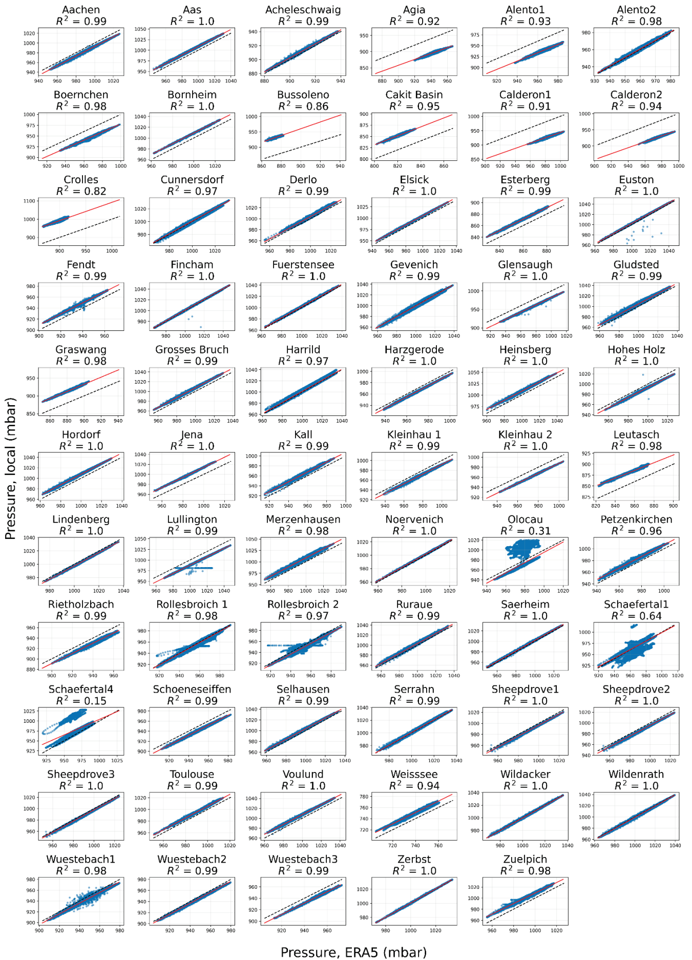
Figure A2: The correlations between atmospheric pressure from local measurements and ERA5 for the COSMOS-Europe sites.
