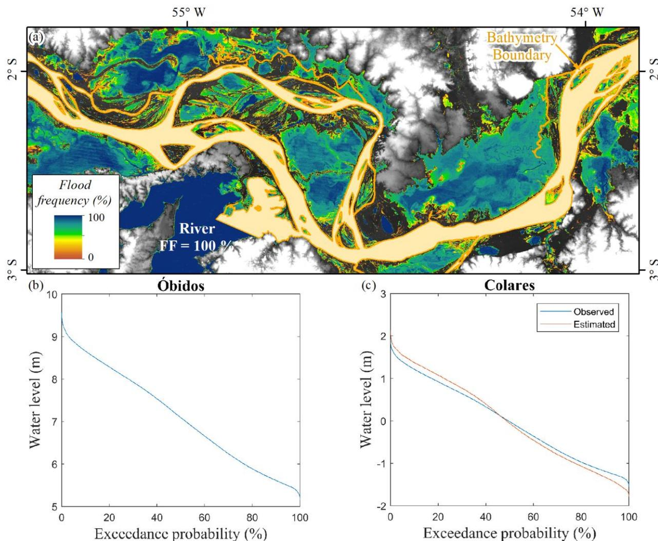
170 **Figure 3.** (a) Close-up view of the flood frequency map over the Amazon estuary's upstream part, (b) Water level duration function at Óbidos station, (c) Water level duration function observed and estimated at Colares station (see Fig. 1 for the location of these two stations).
