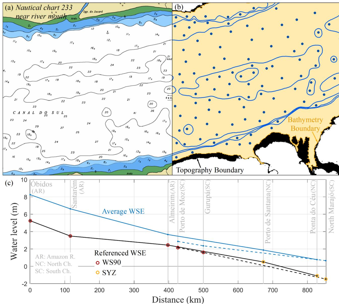
125 **Figure 2.** (a) Example of a nautical chart nearby river mouth (code 233); (b) Digitized pointwise soundings and isobaths, along with bathymetry boundaries (defined as the isoline 96% of flood frequency) and topography boundaries (defined as the isoline 0% of flood frequency); (c) Referenced WSE and Average WSE along the Amazon estuary (EGM08 geoid).
