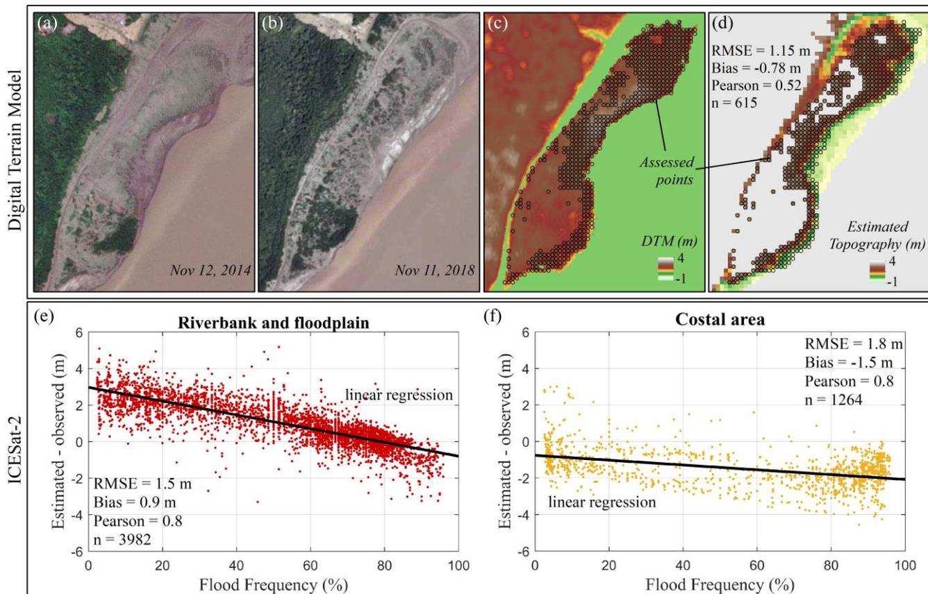
290 **Figure 4.** Sandbank represented by GEA/EB DTM and topography mapping (location in Fig. 1). (a) and (b) represent true-color
