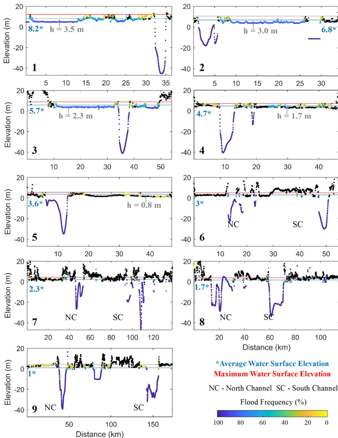
345 **Figure 7. Topographic profiles distributed every 100 km along the river, with the flood frequency, average and maximum WSE, and height between the average level and the minimum elevation of the floodplain.**
