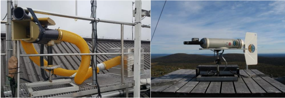
Figure 3. CAPS (left) and FSSP-100 (right) ground setups as installed on the roof of Sammaltunturi station.
