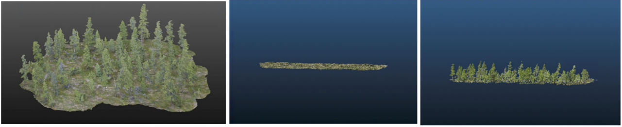
Figure 4: Left: example of a full Red Green Blue (RGB) structure from motion (SfM) point cloud for plot EN18074. Centre: segmented RGB point cloud containing only the points of the ground layer named groundonly . Right: segmented RGB point cloud with the above-ground vegetation named treesonly .
