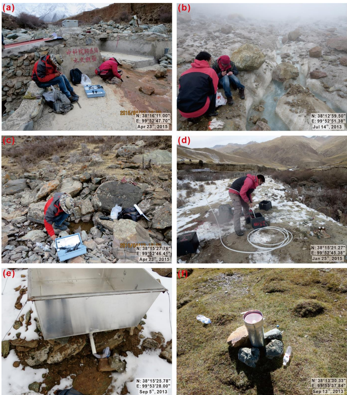
Figure 8. Pictures showing procedures for sampling (a) river water, (b) glacier meltwater, (c) spring water, and (d) groundwater in the field. Devices for collecting snow meltwater and precipitation were shown in (e) and (f), respectively.
