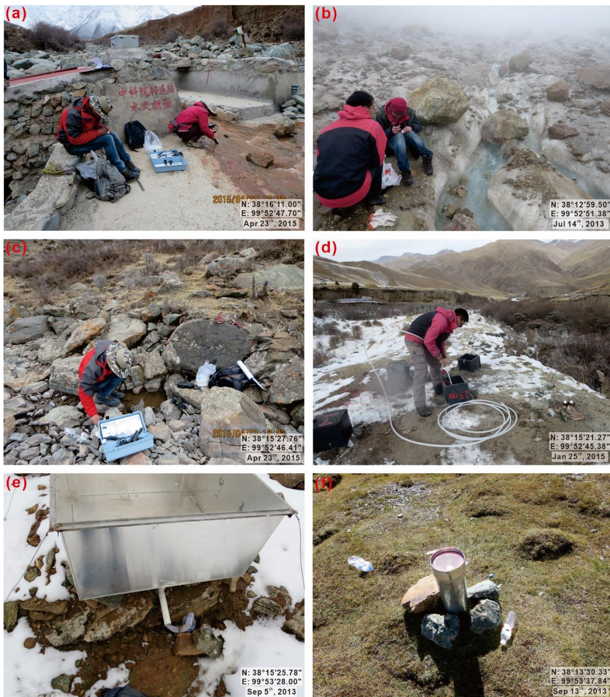
Figure 3. Pictures showing procedures for sampling (a) river water , (b) glacier meltwater, (c) spring water, and (d) groundwater in the field. Devices for collecting snow meltwater and precipitation were shown in (e) and (f), respectively.
