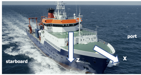
A) Maria S. Merian research vessel and orientation of the reference system
