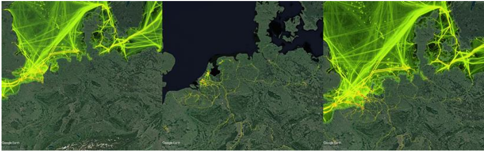
Figure 66 Example emission distribution of CO 2 for sea shipping (left), inland shipping (middle) and sum of both (right) for a specific region covering parts of the North Sea, Baltic Sea as well as inland waterways (example for 2016, at high resolution of 1/60° x 1/120°) (figures using Google Maps)
