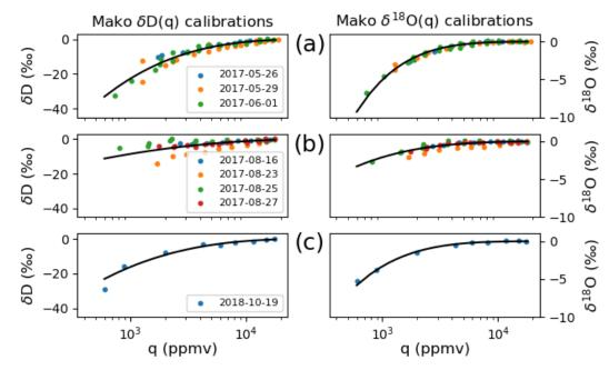
Figure 4: Mako isotope ratio humidity-dependence corrections for ORACLES (a) 2016, (b) 2017, and (c) 2018. Data points are colored by date that the calibration was performed. Fit curves are generated using nonlinear regression with Eqn. 2.
