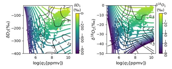
Figure 5: Cross-calibration of Pic2 to Pic1 for the 2017 sampling period. (a): Pic1  $\delta D$  vs Pic2 log(q) and  $\delta D$  (scatter) with model-fit (colored contours). (b): Same as (a) but for  $\delta^{18}O$ . Both fits have  $R^2>0.95$ . Root-mean-squared-errors for q>4 g/kg (where the Pic2 data are most relevant) are 2 % for  $\delta D$  and 0.4 % for  $\delta^{18}O$ . Black contours are model residuals.
